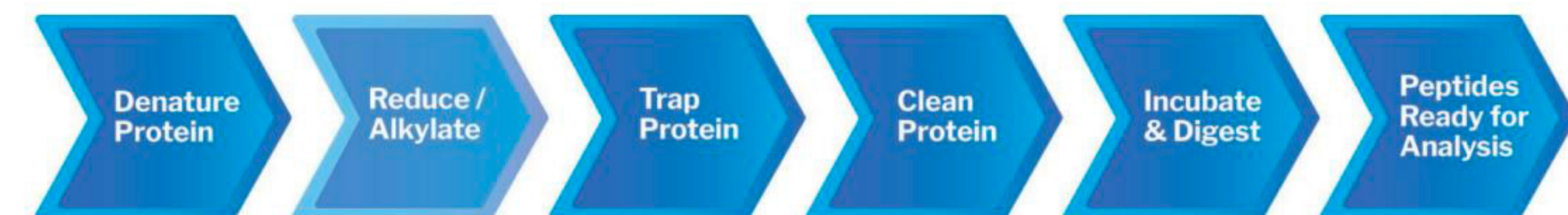
Fig. 1 The 96-well Multi-Attribute Method (MAM) Mini Plate Kit standardizes the rapid analysis of biological medicines at every stage of manufacturing, eliminating the need for protocol development. The kit fully removes a broad range of contaminants including detergents, salts, buffers, stabilizers, excipients and others for samples of 10 µg – 250 µg of biological drug sample. The kit minimizes or eliminates deamidation and chemical artifact formation.
